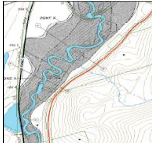
Figure 4.2: This image shows data from the FEMA Flood Insurance Study along the Wells River. The lines crossing the stream channel, indicate that base flood elevation data is available.
